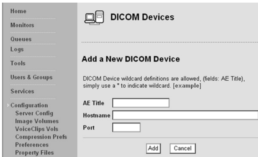
FIG. 2. Screen capture of part of a device table in image management software. Courtesy of integrated PACS provider, Amicas Inc., Boston, MA, www.amicas.com . PACS, Picture Archive and Communication System.
